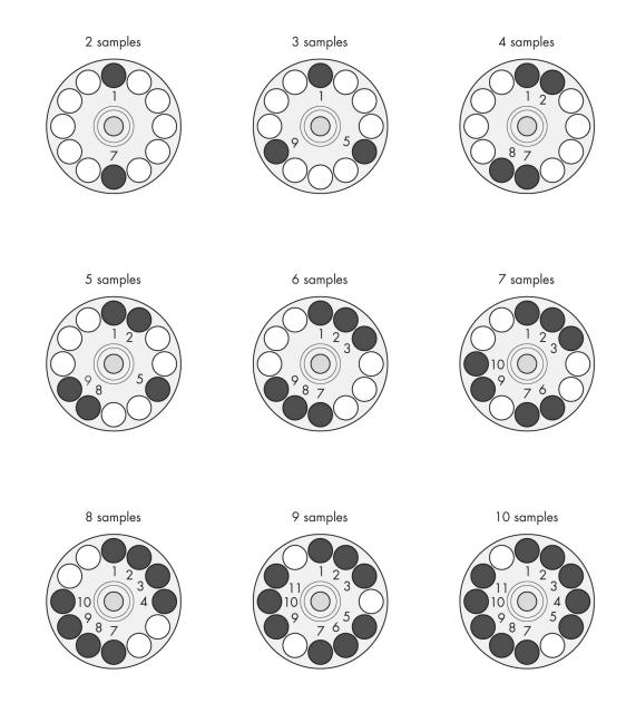
**Figure 1. Loading the TissueLyser LT Adapter.** Ensure that the TissueLyser LT Adapter is balanced by loading samples tubes as shown above.
